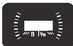
**NOTE:** When the ignition key is out of the STOP position the hourglass symbol is illuminated/blinks to indicate it is recording the hours of tractor operation, regardless of whether the engine has been started.
